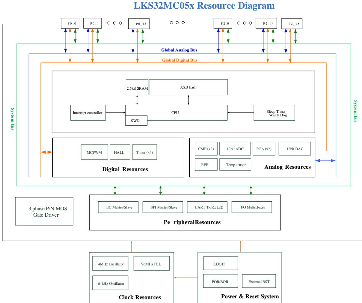
图 1-2 LKS32MC05x with built-in 3P3N driver 系统框图
